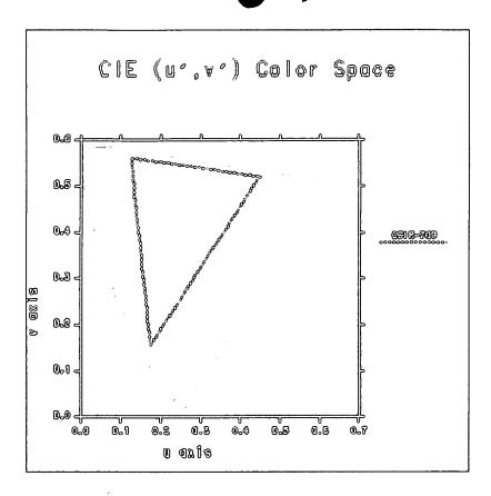
This graph shows clearly that standard color encodings cover only about half of the visible gamut of colors. If future display systems should be able to reproduce this information, it will unavailable from most RGB storage formats. Even existing display systems, since they do not all use the same primary colorants, have significantly varying gamuts, and any restriction on the stored data restricts the reproduction accuracy.
